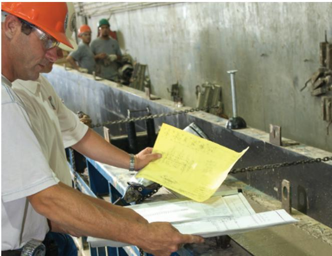
The Precast/Prestressed Concrete Institute's (PCI's) certified auditors compare products against project specifications and minimum requirements as spelled out in the institute's manuals.
